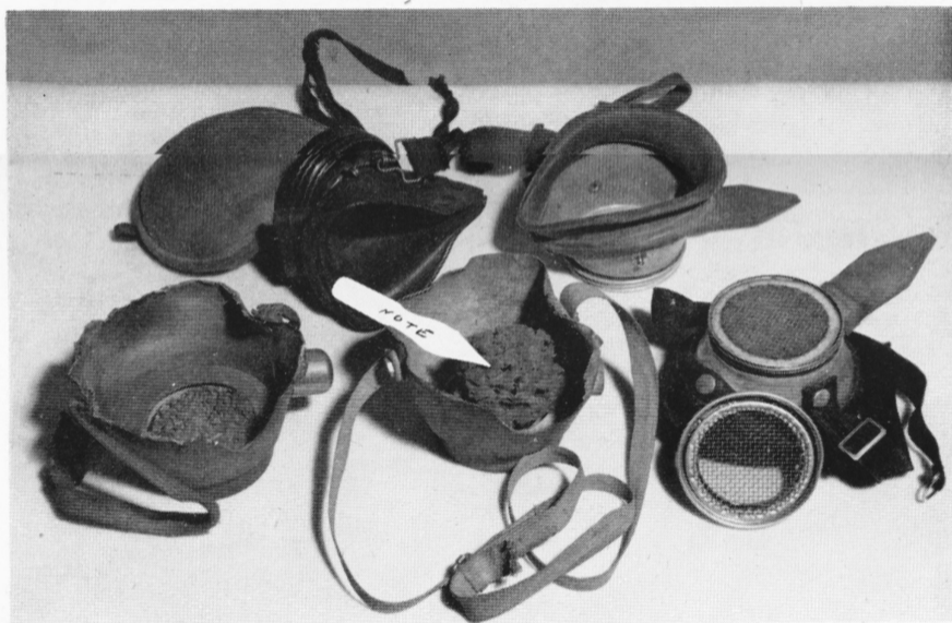
Among the mask-respirators shown in the picture are several old obsolete and useless ones. Note the ones with sponges in the cup. These were turned in recently by a foreman. The rubber is cracked and dry; the valves are gone. They are absolutely useless for protection against dust. New respirators were sent to the department to replace the antiques.
